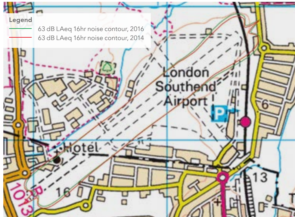
Figure A London Southend Airport summer noise contours 2016. Airborne aircraft noise contours summer average daytime. Contour comparison – 63dB.
