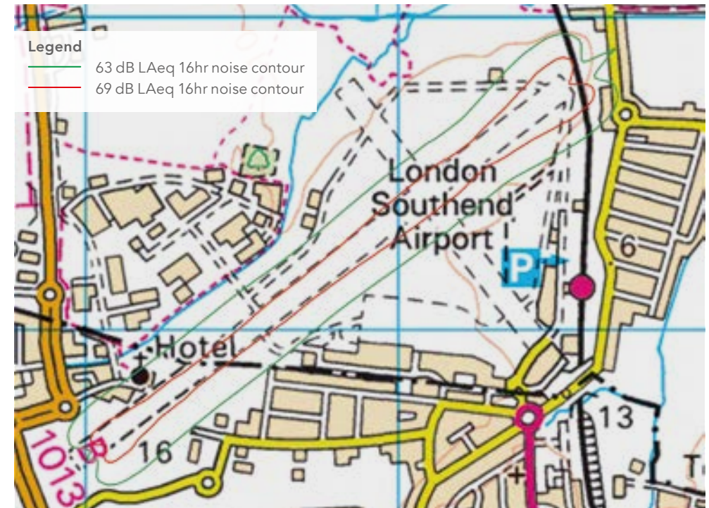
Figure B London Southend Airport summer noise contours 2016. Airborne aircraft noise contours summer average daytime.
